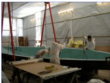
Anticlockwise from left: laminating the first hull for the sailaway; hull joining; and release; the start of the first hull for the kit boat
