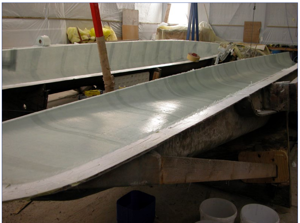
Anticlockwise from left: laminating the first hull for the sailaway; hull joining; and release; the start of the first hull for the kit boat
